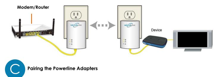
5. Press the **Config Button** for 3 seconds on one Adapter until you see the **Security LED** start blinking **GREEN**. Then press the **Config Button** on the second Adapter until you see the **Security LED** start blinking **GREEN**. The **Security LED** and the **Connection LED** should be solid **GREEN** on both Adapters when they are successfully paired.
