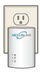
2. Connect this Powerline Adapter to your Modem/Router's LAN Port with an Ethernet (RJ-45) cable. Wait 10 seconds for the **Ethernet LED** to light up **GREEN**, which indicates a connection is established. A flashing **GREEN** light indicates that the device is sending data.
