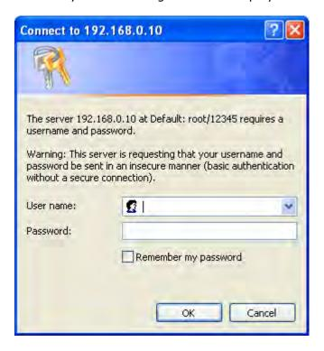
Input the user name and password in the respective fields, default user name is '**root**', and default password is '**12345**', then press the 'OK' button, and you can see the Quick Setup interface of this Wireless-N Powerline Adapter.
