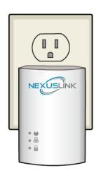
2. Connect this Powerline Adapter to your Modem/Router's LAN Port with an Ethernet (RJ-45) cable. Wait 10 seconds for the **Ethernet LED** He to light up **GREEN**, which indicates a connection is established. A flashing **GREEN** light indicates that the device is sending data.
