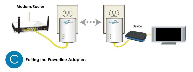
5. Press the **Config Button** for 3 seconds on one Adapter until you see the **Security LED** for start blinking **GREEN**. Then press the **Config Button** on the second Adapter until you see the **Security LED** for start blinking **GREEN**. The **Security LED** for and the **Connection LED** for should be solid **GREEN** on both Adapters when they are successfully paired.
